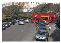
**Photo 4**: Bus swings wide into opposite lane at pedestrian access gate.
